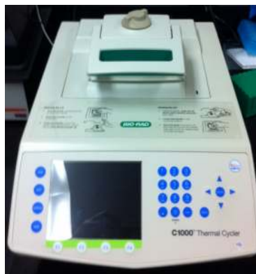
Figure 7. The thermal cycler is used to carry out PCR reaction. Image by Walter Suza.
